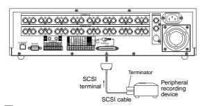
When connecting a peripheral recording device, the SCSI TERMINATION switch must be set to OFF.
